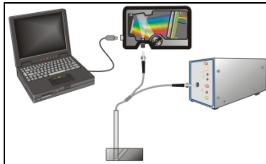
Figure 6-3: Typical reflection setup. A light source (far right) sends light via the input leg of a reflection probe onto a sample (bottom center). A reflection probe holder holds the probe in either a 90 or 45-degree angle from the surface. The output leg of the reflection probe carries light from the sample to the spectrometer (top center), which is connected to the PC (far left).
